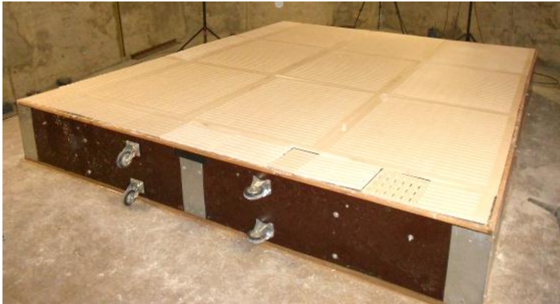
Figure 2: Bailey Interiors Justice Panel 1200mm x 1200mm Perforated Plaster Ceiling Panels with 50mm thick 32kg/m 3 Glasswool installed to rear of panels tested with a 400mm air gap installed into the Reverberation Chamber for testing.
